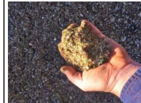
Crushed glass sand produced by Lismore City Council
