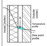
This shows a wall with a higher air temperature inside than outside. The temperature profile (solid line) is below the dew point profile (dashed line) in the coloured region, X. When the surface temperature is below the dew point in this region, condensation is likely to form on surfaces within it.
