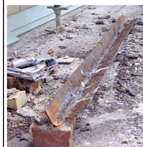
This lintel was revealed during building work on a structure 200 m from salt water and within 2 km of breaking surf.
