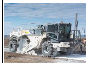
In situ mixing of binders
