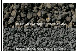
10 mm and 20 mm blue metal aggregate comparison
